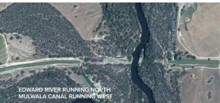
Deniliquin's irrigation system also receives water from the Mulwala Canal. This large water system runs 160 kilometres west from Lake Mulwala to Deniliquin. The canal is often referred to by irrigators as their 'man-made river'.
